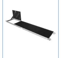
Pass-by platform with flap: 2.85 x 0.61 m Weight: 20.28 kg Platform with flap made of aluminium frame lined with multi-ply water resistant plywood of antislip surface. Provides free inter-storey communication. Attached to frame rung with catch pawl.
