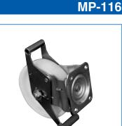
Castor: 200 mm diameter Weight: 3.95 kg 200 mm diameter castor used as the set with footing with two nuts MP-114 or MP-138. Useful load of one castor equals to 750 kg. The castor is equipped in foot brake.
