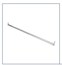
Horizontal transoms for different field length made of pipe of 48.3 mm diameter. Transoms constitute stiffening elements of scaffolding construction and protective railings and in case of platform wooden balks they serve as the supporting elements. Specially profiled bits with incorporated wedges are installed at both transom ends. The wedge is hammered on the plate aperture disc.
