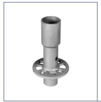
Primary element with plate having apertures for fastening horizontal transoms E3718xx. The element is installed on threaded spindle of footing for levelling purposes of the lowest scaffolding storey and is used for vertical stands E3714xx positioning. It also serves as the scaffolding expanding element.
