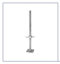
Footings of different heights used for levelling the ground slips. Foot dimension 150 x 150 mm with threaded pipe plunger, nut and socket for steel frame pipe. Hammered thread protects against screwing out of the nut (there must be at least 15 cm of threaded plunger in the frame) and its loss. Footing height 40 cm, max. screwing out length — 25 cm; footing height 60 cm, max. screwing out length — 65 cm. Footing permissible loading equals to 3 t and depends on height of nut undoing.
