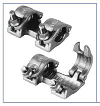
Used for coaxial, in-line connection of two pipes of 48 mm diameter. The in-line coupling must be made with aligning pin fixed in the contact point of two pipes. Permissible load of in-line coupling equals to 6 kN.
