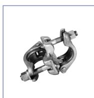
Fixed in the field of stiffening sheet with anchor coupling and is used for anchoring of scaffolding to the object. With flange nuts, used for connection of two pipes of 48 mm diameter at angle of 90 degrees. Permissible load of normal coupling amounts to 9 kN.
