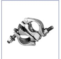
Supplied with flange nuts is used for connection of two 48 mm diameter pipes at any angle. Permissible load of rotary coupling amounts to 5 kN.
