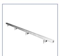
U-profile for 2, 3, 4, 5, 6 platforms 0.32 m wide and corresponding girder length of 3 m, 4 m, 5 m, 6 m. Fixing to the top belt of girder by the coupling. Used for platforms building of different dimensions
