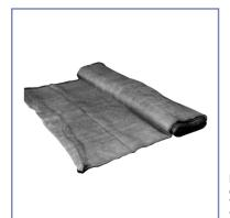
Protecting net screen reinforced with black yarn. Holes situated every 10 cm on whole length for fastening purposes. Weight (G.S.M.) – about 65 g/sqm. Wind transmittance – 50-55 per cent.
